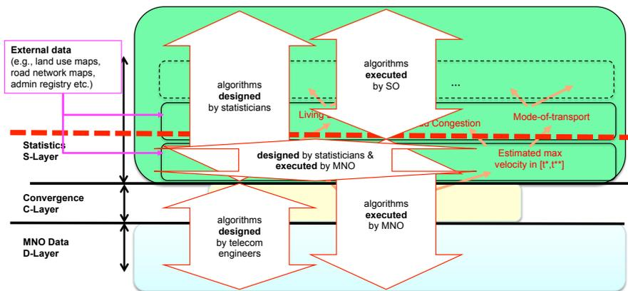
Figure 4: Segmentation in the processing design vs. execution. The bottom part of the S-layer still includes individual micro-data and is executed within the MNO domain. Intermediate aggregate data (non-personal) that are produced within the S-layer are then exported to the SO.
