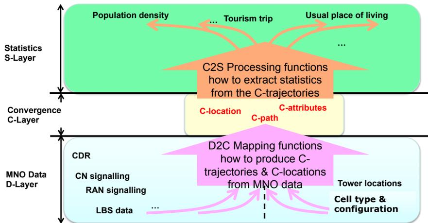
Figure 3: Decoupling of D2C and C2S functions.
